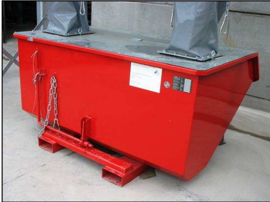
Dual tipping container with flexible attachments to minimise forklift damage during removal.
