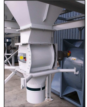
Rotating valve with big bag support.
