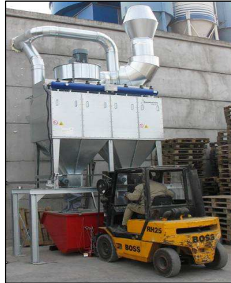
Dual tipping container with flexible attachments to minimise forklift damage during removal.
